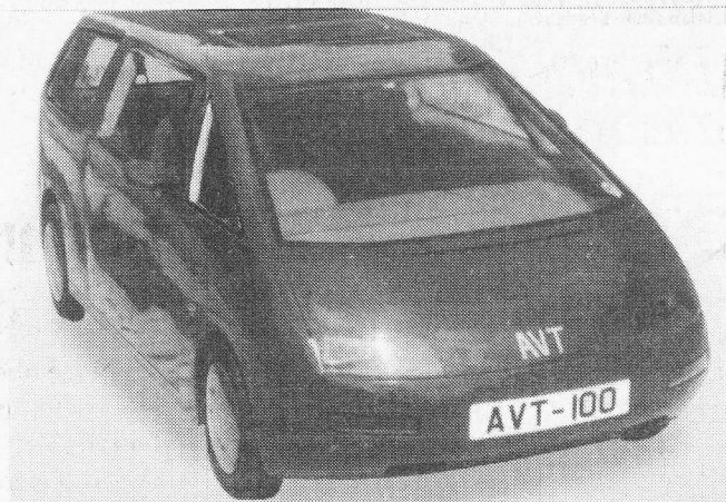
The composite-bodied AVT-100 uses regenerative braking. Top speed is 80 mph, range is 60 miles.
