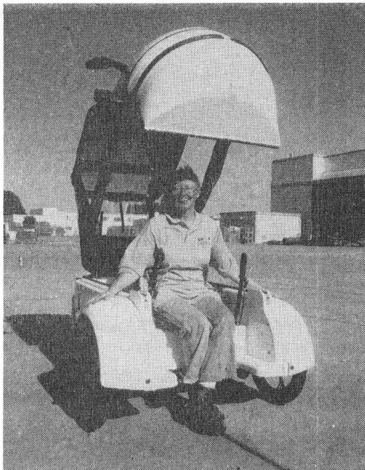
Gizmo's Flip-up nose and canopy provides easy access you just sit down and the car closes around and over you.
