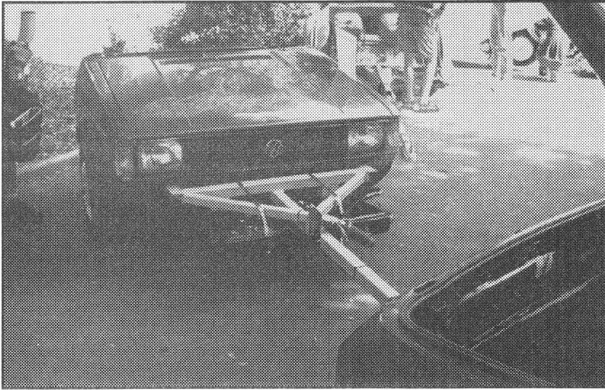
Something new for SV Rally 2000 was JB Straubel's Pusher. Unlike a generator APU the trailer pushes the EV.
