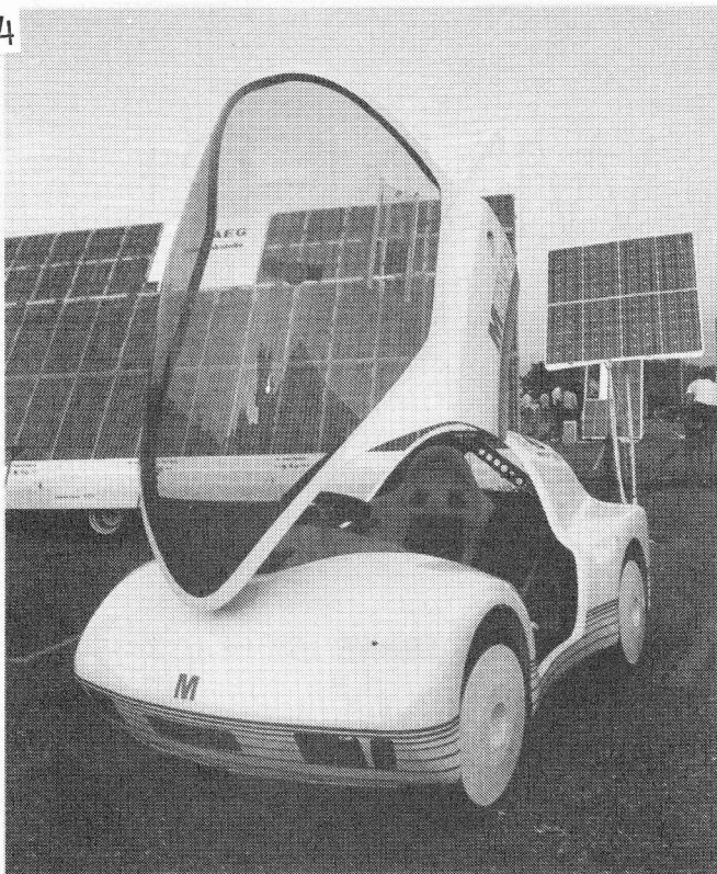
MEV1 with mobile solar cell panel
