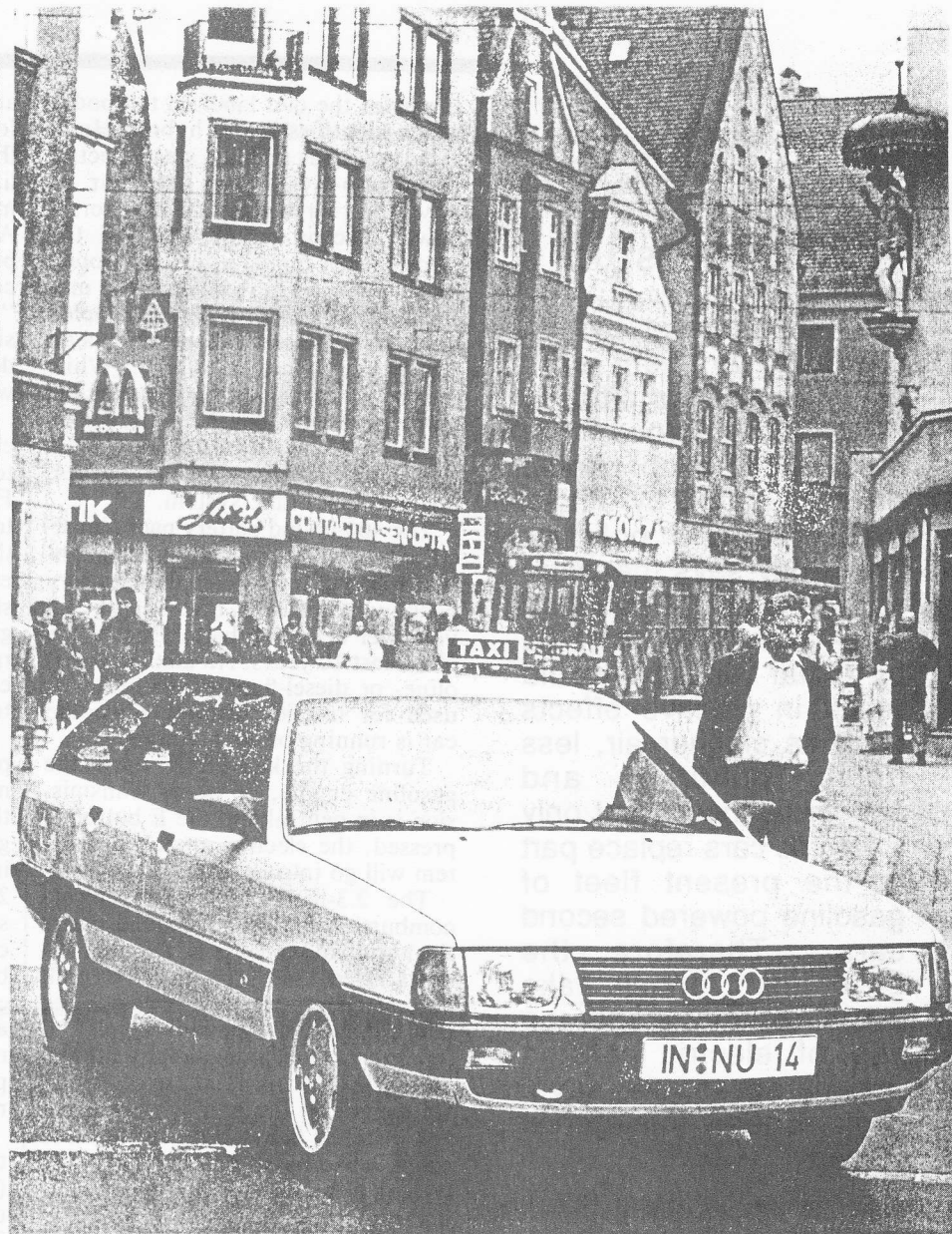
Audi duo. The duo, a modified Audi 100 Avant Quattro, uses a gasoline engine to drive the front wheels and a small electric propulsion system to drive the rear wheels.
